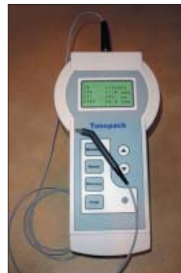
The TonoPach™ measures both applanation determined intraocular pressure (IOP) and central corneal thickness (CCT) at the same locus on the cornea. The display on the TonoPach indicates conventionally measured IOP, CCT and corrected IOP.
